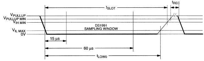
$\begin{array}{l} 60 \ \mu s < t_{LOW0} < t_{SLOT} < 120 \ \mu s \\ 1 \ \mu s < t_{REC} < \infty \end{array}$
